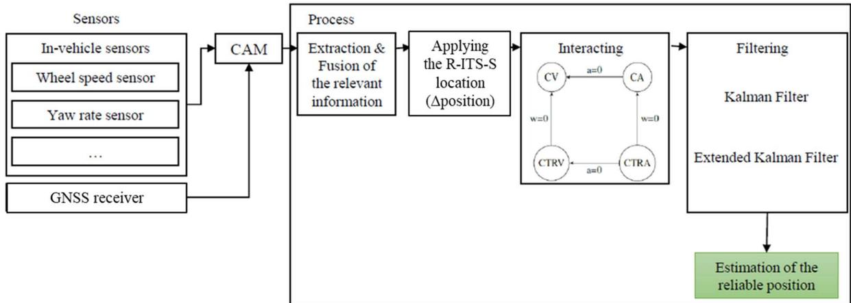
Figure 10: Global view of the geolocation method
