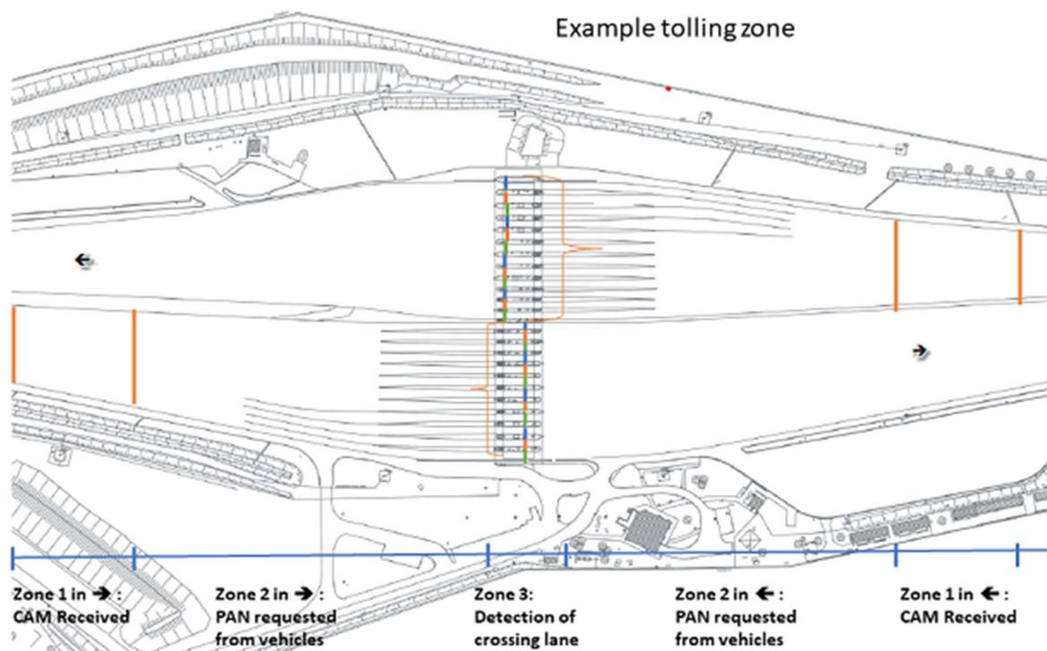
**Figure 8: Zones used during vehicle geolocation**
