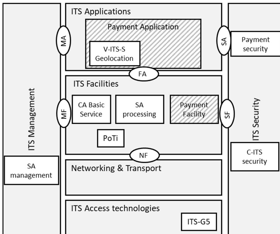
**Figure 26: ITS-Station Architecture for payment applications**
