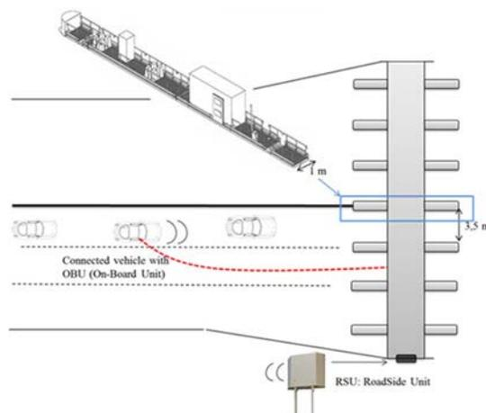
**Figure 7: Possible ETC system using R-ITS-S equipment**
