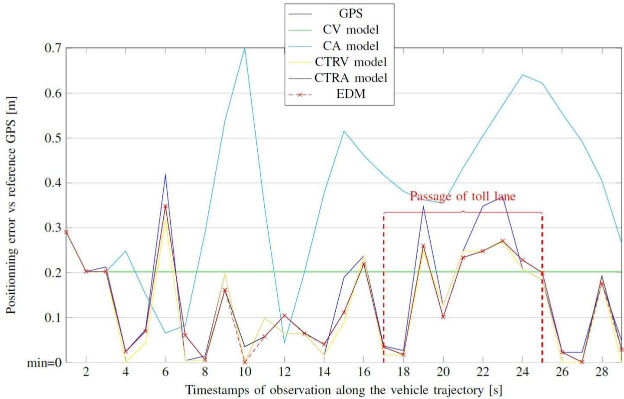
**Figure 20: Evolution of the errors compared with the reference trajectory while passing the toll plaza**
