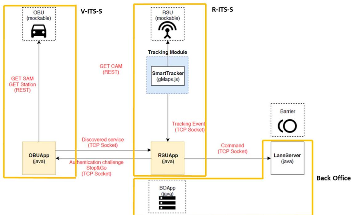
Figure 16: Architecture of the testing modules of the electronic toll application in C-ITS
