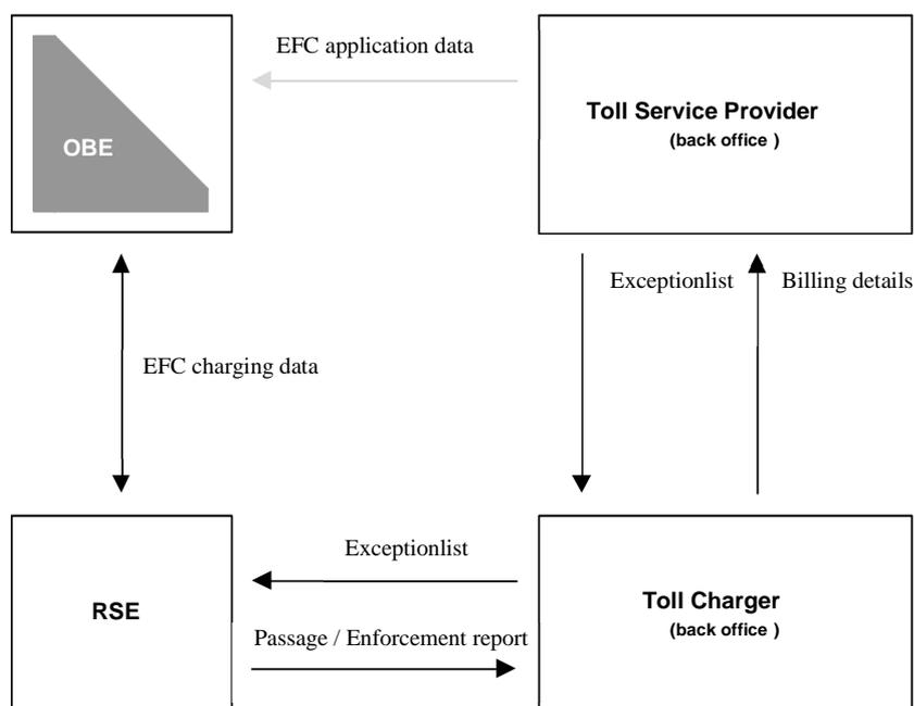
**Figure A.3: Technical architecture for infrastructure-based EFC systems (see also [i.34])**
