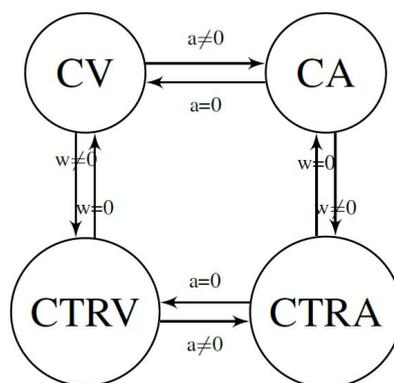
**Figure 12: Transitions between vehicle motion state by setting one variable to zero**
