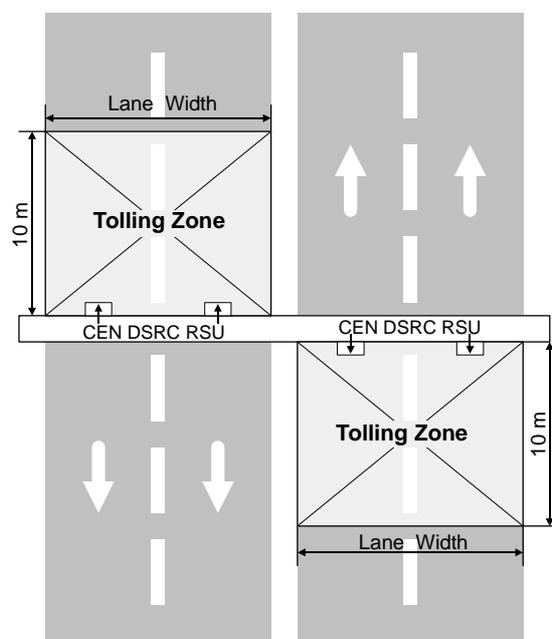
**Figure 6: Typical tolling zone geometries for a two-lane free flow scenario**
