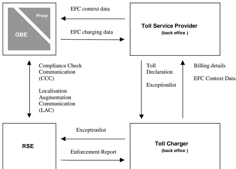
**Figure A.4: Technical architecture for Autonomous EFC systems (see also [i.34])**
