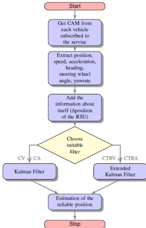
Figure 11: Loop process as long as the R-ITS-S (noted as RSU) receives CAM from the subscribed vehicles
